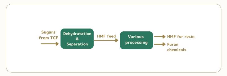
HMF produced in this manufacturing line will be tested as a formaldehyde replacement in the production of Engineered wood. In particular, Medium Density Fibreboard (MDF) and plywood for interior usage. Furthermore it will be used as a starting point for the production of different furan-based green products.
